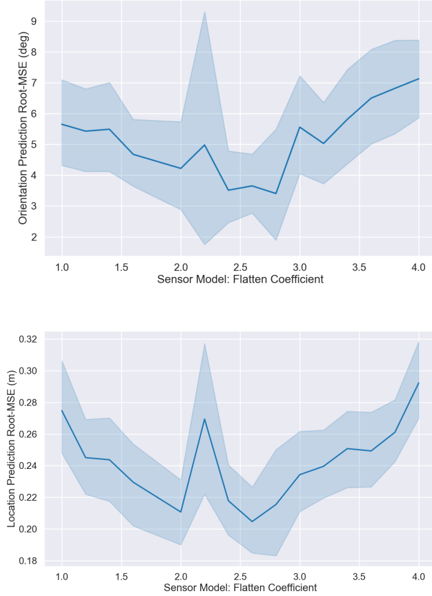
Figure 7: The particle filter performance in the 2D simulation with varying flatten exponent denominators. Performance is measured as root-mean-square error in position and orientation.
