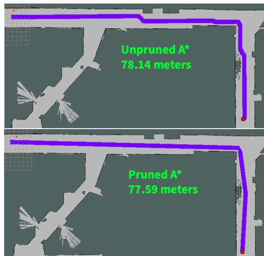
Figure 3: An example of pruning nodes. The pruned trajectory is slightly shorter as a result of taking a more direct path. With fewer turns, the pruned path is also easier for pure pursuit to follow.
